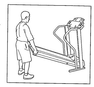
Move your right hand to the position shown and hold the treadmill firmly. Raise the treadmill until the frame passes the storage latch. Make sure that the storage latch is inserted into the slot in the side of the frame.
